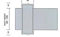
Overall width of installation frame is = Duct width + 116mm
